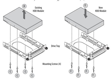
6. Install the new HDD module to the tray.
