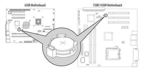
The battery must be replaced during the life of the computer. Battery life depends on the amount of time the computer is on, or on-time.
