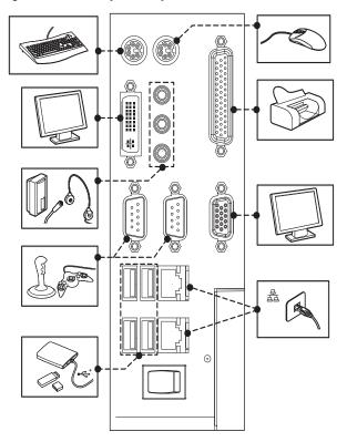
Figure 20 - 750R and 1450R Computer Peripherals
