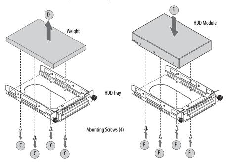
**5.** Install the new HDD module to the tray.
