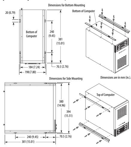
Figure 18 - Mounting Dimensions for 750R Computer
